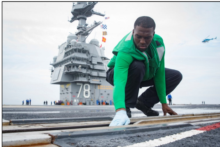
Aviation Boatswain's Mate Third Class Darius Harmon lubricates the EMALS on the Gerald R. Ford 's flight deck.
